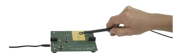
Detection of emitted interference - RF-E 05 E-field probe via demonstration board SA 21  $\,$
