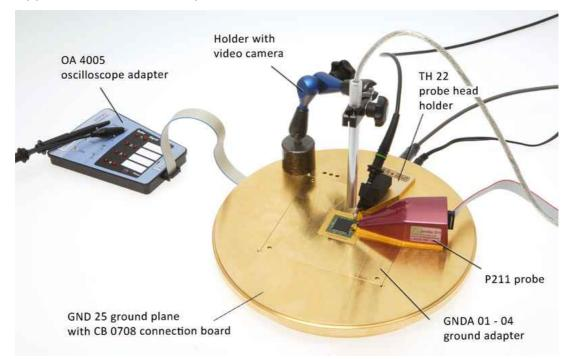
Scheme measurement set-up Set ICE1 with extern devices
