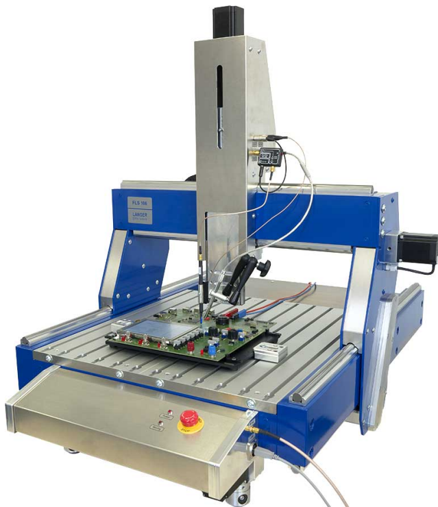
FLS 106 application with board, near-field probe and microscope camera
