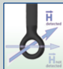
Magnetic field measurement: RF-R 50-1 In the vicinity of modules and on larger components, up to a distance of 3 cm
