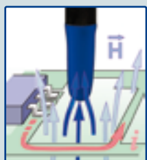
Magnetic field measurement: LF-B 3 Directly on modules, detection of critical current loops in the layout
