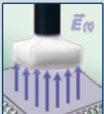
E field measurement: RF-E 09 At a distance of 0.5 mm to 10 mm on the surface of multi-pin ICs and electronic modules
