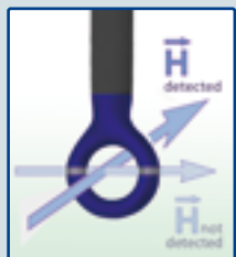
Magnetic field measurement: LF-R 50 At assemblies, devices or cables up to a distance of 3 cm, larger components as potential weak points
