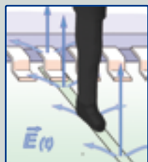
E field measurement: RF-E 05 Directly on modules or wide conducting paths
