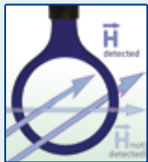
Magnetic field measurement: LF-R 400 Up to a distance of 10 cm around assemblies and devices
