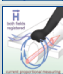
RF current measurement: RF-U 5-2 At wide conducting paths, cables, connectors, electronic components and their connections - Works like a coupling clamp
